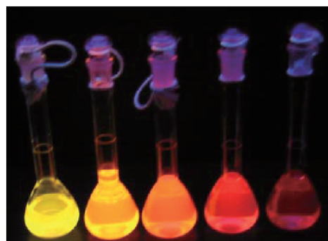
Figure 4. Fluorescence images of 2 in cyclohexane, toluene, THF, dichloromethane, and DMF (from left to right) under UV light irradiation.
